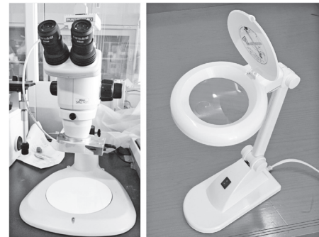
Fig. 2 Left; Stereo microscope. Binocular observation is possible under ring, shadow less, illumination, Right; Loupe with LED ring lighting used in K mold method used before casting in this report.
